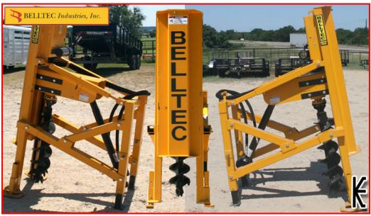
Frame-Guided Auger System Twin hydraulic cylinders connect the auger carriage to the mainframe of the machine. The cylinders move the carriage up and down the mainframe slides. Adjustable feet on the mainframe may be leveled. Since the auger is guided into the ground by the mainframe, as long as the mainframe is straight and the carriage is level, the machine will drill straight holes.
